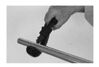
**Step 2**De-burr the internal and external tube ends.
