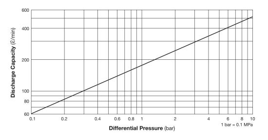
1. Differential pressure is the difference between the inlet and outlet pressure of the air vent. 2. Capacities are equivalent capacities of air at 20°C under atmospheric pressure.
