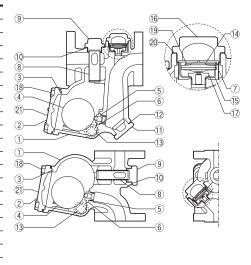
Replacement kits available: (M) maintenance parts, (R) repair parts, (F) float
