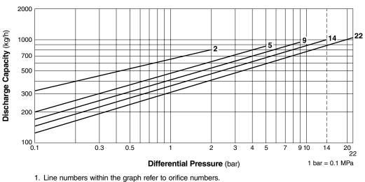
2. Differential pressure is the difference between the inlet and outlet pressure of the trap. 3. Capacities are based on continuous discharge of condensate 6 °C below saturated steam temperature.
