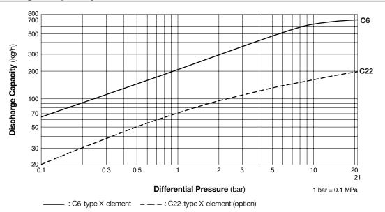
Differential pressure is the difference between the inlet and outlet pressure of the trap.
