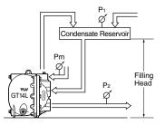
The discharge capacity is determined by the motive medium, motive medium pressure (Pm) and back pressure (P2).
