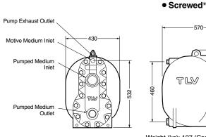
Weight (kg): 127 (Cast Iron), 139 (Cast Steel) \* BSP DIN 2999, other standards available
