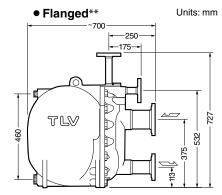
Weight (kg): 149 (Cast Steel) \*\* DIN 2501 PN 25/40, ASME Class 150 RF, other standards available
