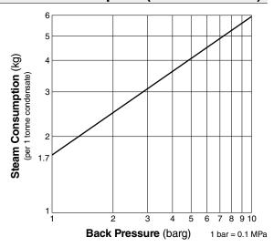
Capacity of GT14 as a steam trap (P<sub>1</sub> > P<sub>2</sub>). Instantaneous condensate loads above the rated trap capacity will cause the pump to cycle and therefore reduce the discharge capacity.
