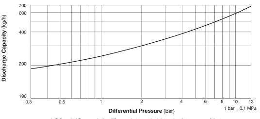
1. Differential Pressure is the difference between the inlet and outlet pressure of the trap. 2. Recommended safety factor: at least 2.
