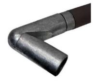
Made of ductile iron HDG Galvanised finish (BS EN ISO 1461:2009) Suits 1 1/4" (42.4mm) OD steel pipe Installation with 8mm Allen key
