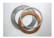
**Taylor ring gaskets** are manufactured from thin sheet metal formed into embossed concentric rings. Taylor ring gaskets may be used with jointing compound or with cord cemented into the corrugations. **Taylor ring gaskets** are essentially line-contact gaskets with the corrugations providing mechanical support to the compound or cord filling. The resilience of **taylor ring gaskets** depends on the type and thickness of the metal used as well as the pitch and depth of the corrugations.
